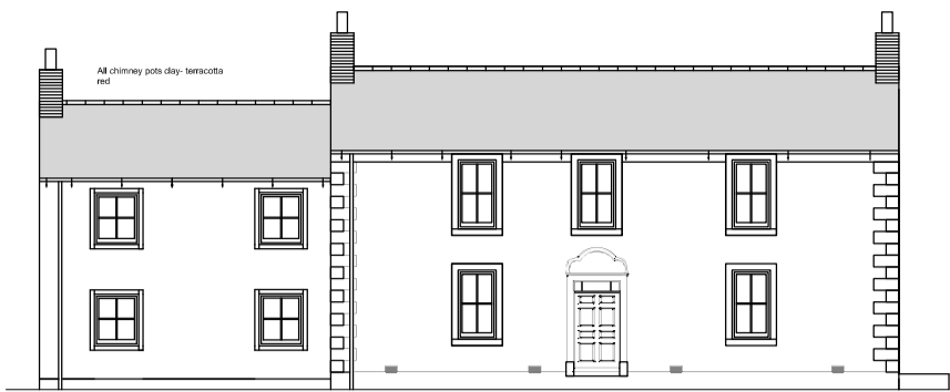
FRONT ELEVATION Following render repairs - restate rose render band to window surround
