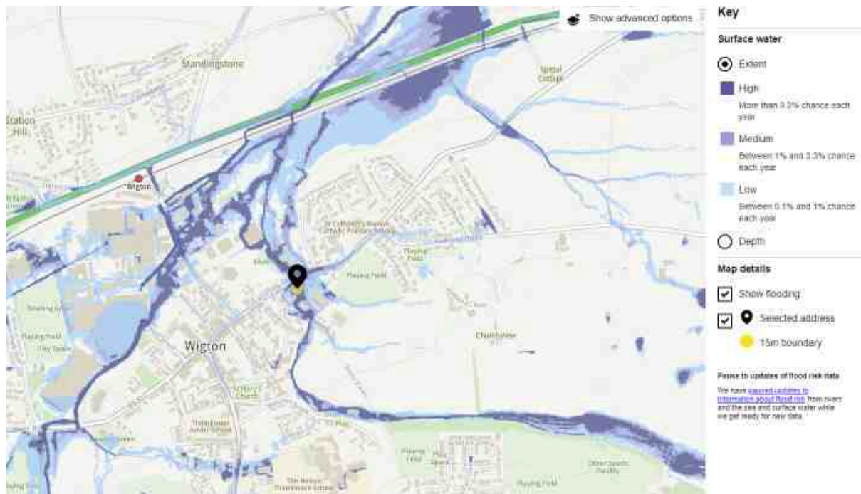
Figure 2 - Surface Water Flood Extent
